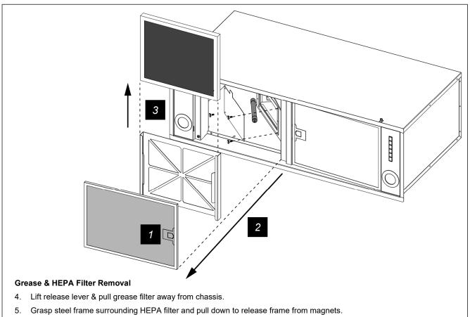
6. Slide the HEPA filter sideways away from the HEPA filter frame.
