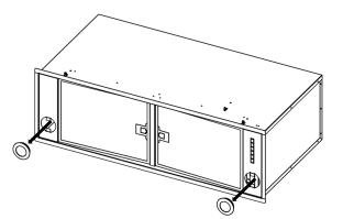
The long-life LED Lamps can be replaced as follows; Pull the lamp from behind to separate from the extractor body. The lamp should be unplugged and replaced with the new lamp. Connect the new lamp plug socket and push the new lamp into place (which will be retained in position once the back of the lamp body meets with the extractor surface). Only lamps supplied by Westin should be used. In the event of any difficulty please call Westin.
